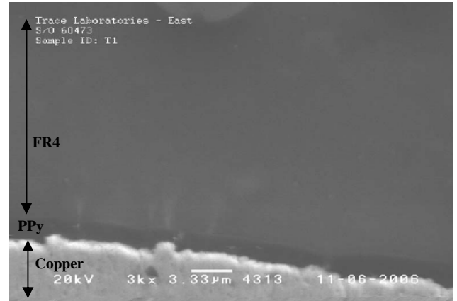
Figure 6 Group B specimen (representative cross-section view)
